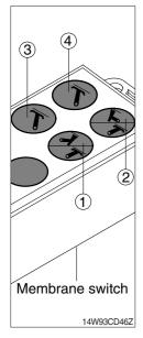
(1) This switch is used to select dozer blade or outrigger operation.
